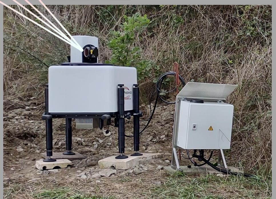
Halo Photonics Stream Line<sup>XR</sup> Scanning Doppler LIDAR
